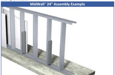
Midwall™ 24" is generally used in interior half walls of less than 48" in height. Attach Midwall to 54 mil stud with #12 screws through all pre-drilled guide holes. Other studs in the wall are typical infill studs.
